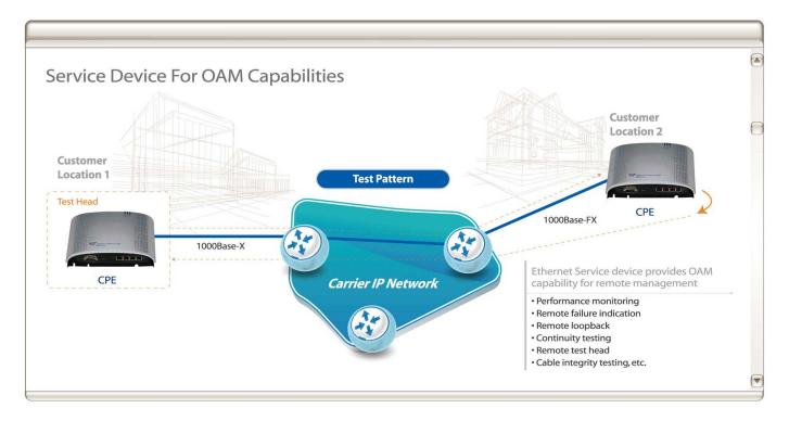
operator receives notification of equipment outages. In the event of a fault, the information generated by OAM helps the operator troubleshoot the network to locate the fault, identify which services have been impacted, and take the appropriate action.
