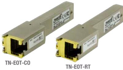
The TN-EOT-xx Series is an Ethernet Extender in a standard SFP form factor, it provides the ability to leverage the existing 2-Wire or Coax cable infrastructure to extend the Ethernet service. It can extend the Ethernet service on 2-wire with distances up to 400 meters at 200Mbps bi-directional data rate or extend Ethernet on Coax cabling with distances up to 500 meters at 300Mbps bi-directional data rate.
