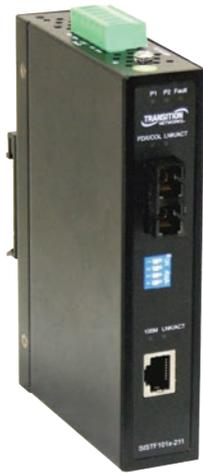
The SISTF Series is an unmanaged hardened Fast Ethernet media converter supporting multimode or single mode fiber connections with SC or ST connectors for extended distance communications up to 30 kilometers. These converters are Class 1, Div 2 Certified, have redundant input power connections, and a fault alarm relay to ensure safe reliable operation in temperatures between -40°C and +75°C.
