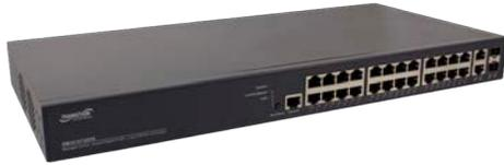
This switch is a high performance Layer 2 managed switch with 52Gbps switching capacity. It provides (24) 10/100/1000Base-T copper ports with IEEE 802.3at PoE+ capability and (2) additional 100/1000 dual speed SFP/RJ-45 Combo ports.
