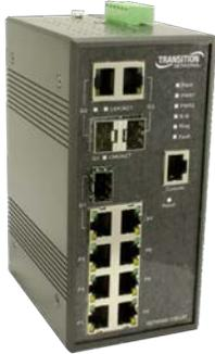
The SISTM1040-173D-LRT is a hardened managed switch in a rugged enclosure used at the edge of a hardened network to provide Fast Ethernet connections. This switch has (7) 10/100Base-TX ports and (3) combo Gigabit RJ-45/SFP ports. The SFP slots will accept 100MB or Gigabit SFP modules to provide multimode or single mode fiber communications.
