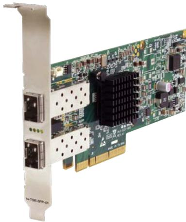
The N-TGE-SFP-01 is a 2-port PCIe bus fiber NIC that supports a 1Gbps/10Gbps link. The open SFP slots can be used with 1000Base-X SFPs or 10GBase-SR/LR SFP+ modules. The NIC fully complies with IEEE 802.3ae and IEEE 802.3z standards. It provides up to 20 Gbps full-duplex bandwidth capacity to support high-end servers. It is suitable for data center, SMB and Cloud computing applications. Two LED indicators (LINK and ACT) on the bracket will help to oversee the board link and activity status.
