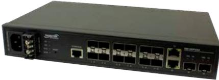
This switch is a next generation fully managed fiber switch with 68Gbps switching capacity. It provides (12) 100/1000 dual speed SFP slots, (2) 1G/10G SFP+ slots and 2 additional Gigabit RJ-45 ports.
