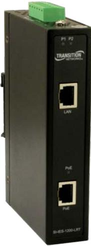
The SI-IES-1200-LRT is an unmanaged hardened PoE+ injector that adds up to 30 Watts of power on a network segment. Injectors are commonly used to power PoE devices in locations where a power source does not exist. The injector has redundant input power connections, and a fault alarm relay to ensure safe reliable operation in temperatures between -40°C and +75°C.
