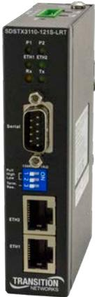
Transition Networks hardened serial device server provides the ability to communicate secured serial data across an Ethernet network. The SDSTX3110-121S-LRT contains two 10/100 Fast Ethernet ports that can be configured to communicate to one or multiple redundant servers. Security of the data transmission is assured through HTTPS, SSH, and SSL data encryption.
