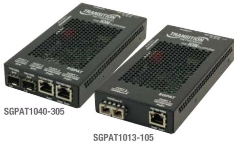
The SGPAT Series is a 10/100/1000Base-T to 1000Base-SX/LX Gigabit Ethernet Media Converter, that easily and affordably facilitates the connection between different types of network cabling, while also injecting PoE+ power through the copper RJ-45 port.
