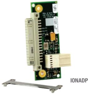
The IONADP is an adapter card that allows the ION Platform chassis to be backwards compatible with Point System™ modules. This adapter is designed to sit between a Point System™ module and the backplane of the ION chassis. The purpose of the IONADP is to lengthen the Point System™ module so it can be securely mounted in an ION chassis while also connecting to the backplane allowing the ION chassis to power the Point System™ module.
